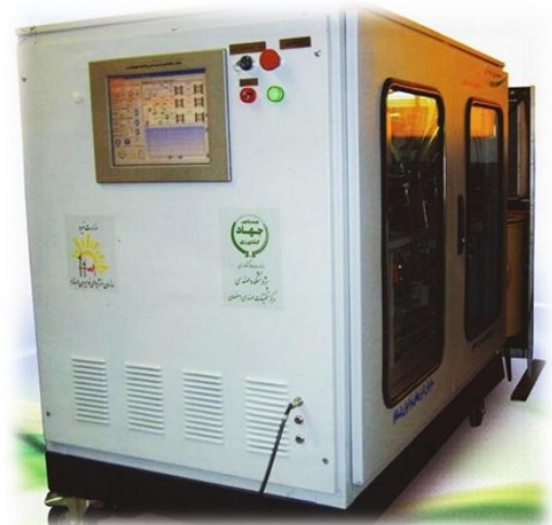
5 KW polymer fuel cell manufactured by Isfahan Engineering Research Center
