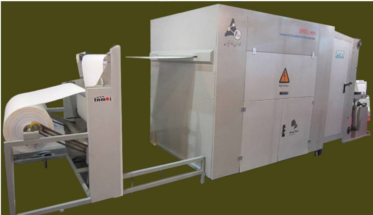
Industrial Electroris Machine for the production of large scale nanofiber filters
